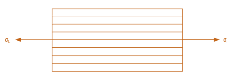
Figure 3.3 Longitudinal loading condition
