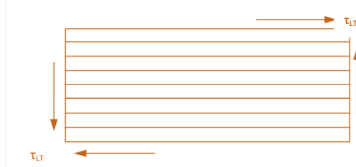
Figure 3.5 Shear loading condition
