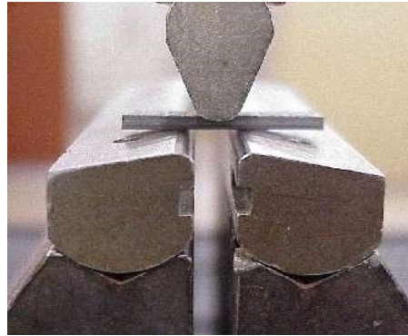
Figure 3.18 Short beam shear test
